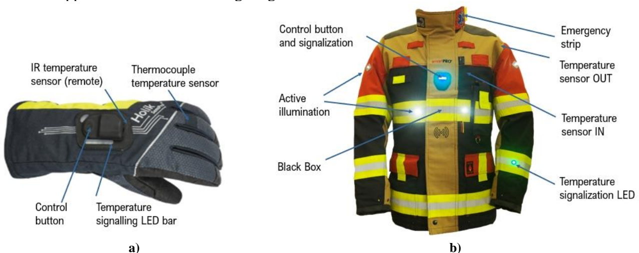
Figure 1. Possible applications a) smart protective glove SensPRO with contact and contactless temperature measurement b) smart protective firefighter suit smartPRO
